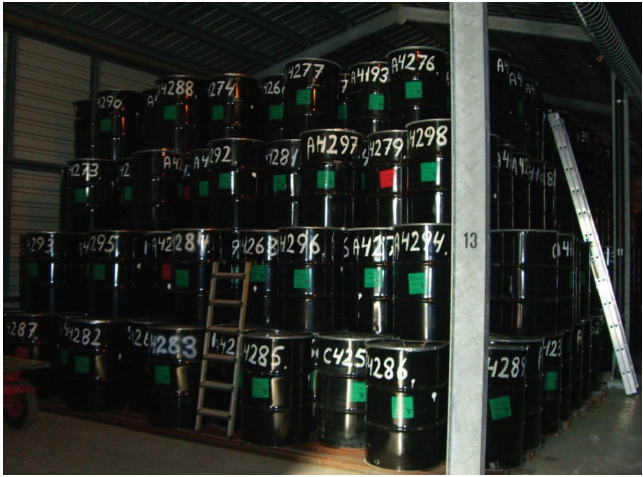
A) 210 liters concrete-lined steel drums
